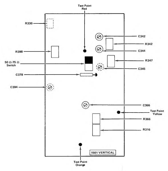
Figure 2-2. Vertical deflection circuit board showing location of test points and adjustable components. Dotted lines indicate locations of components on the left side of the board. The board is mounted in a vertical plane near the DISPLAY OFFSET control.
