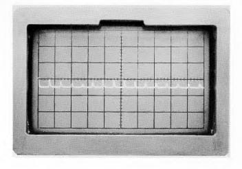
Figure 2-18. 1  $\mu$ s markers at 500 feet/Div; POLY dielectric.
