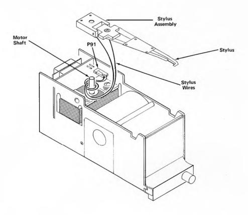
Fig. 3-5. Correct alignment of stylus assembly connecting wire.
