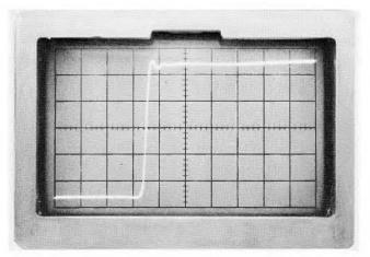
Figure 2-6. Acceptable overshoot and ringing with proper termination.
