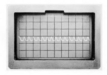
Figure 2-13. 0.1  $\mu s$  markers at 50 feet/Div; POLY dielectric.
