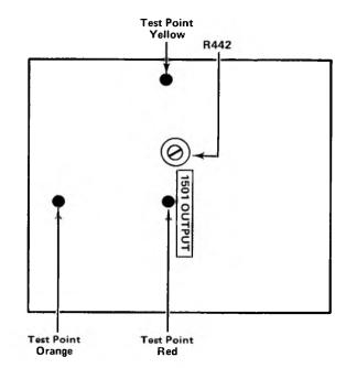
Figure 2-5. Output circuit board showing test points and gain adjustment R442. The board is mounted on a vertical plane directly behind the front panel power switch.
