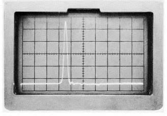
Figure 2-10. Baseline aberrations minimized and amplitude adjusted for 5 divisions
