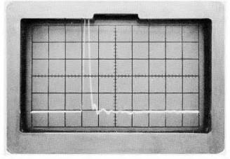
Figure 2-9. R347 adjusted too far clockwise, leading edge moves to the left past the region of the "foot".
