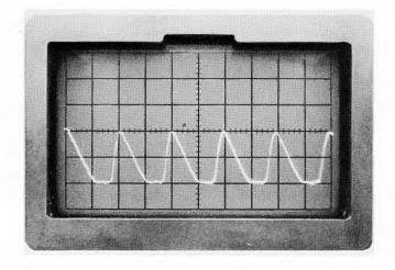
Figure 2-24. 0.1  $\mu s$  markers at 5 meters/Div; POLY dielectric.
