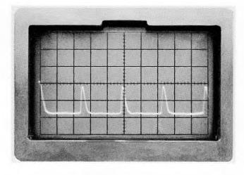
Figure 2-23. 0.5 μs markers at 20 meters/Div; POLY dielectric.
