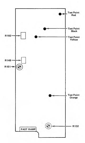
Figure 2-11. Fast Ramp circuit board. Located under and behind the START pushbutton. Mounted in a horizontal plane upside down. R132 is near the START pushbutton. R192 and R148 may be adjusted through holes in the right side panel.
