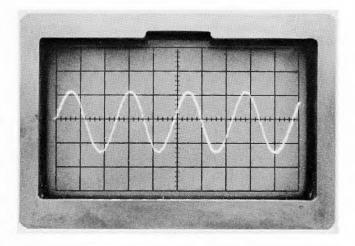
Figure 2-25. 50 ns markers at 2 meters/Div; POLY dielectric.
