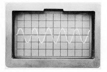
Figure 2-26. 10 ns markers at .5 meters/Div; POLY dielectric.
