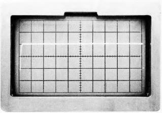
Figure 2-4. Capacitor C394 correctly adjusted.
