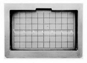
Figure 2-17. 1  $\mu s$  markers at 200 feet/Div; POLY dielectric.
