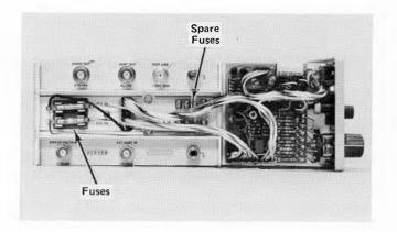
Fig. 3-1. Location of AC line fuses.
