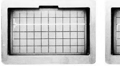
Figure 2-3. Capacitor C394 improperly adjusted.
