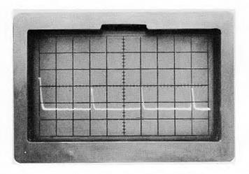
Figure 2-21. 5  $\mu s$  markers at 200 meters/Div; FOAM .81 dielectric.
