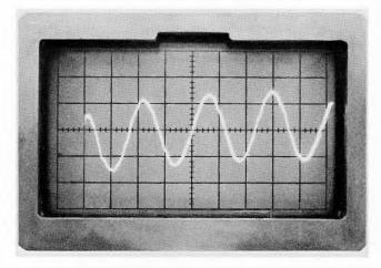
Figure 2-28. 50 ns markers at 2 meters/Div properly positioned for setting of 000 on the START POINT control.
