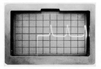
Figure 2-27.  $0.5~\mu s$  markers at 20 meters/Div properly positioned for setting of 000 on the START POINT control.
