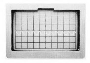
Figure 2-12. 0.1  $\mu$ s markers at 50 feet/Div; AIR dielectric.
