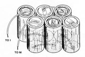
Fig. 3-3. Connection of battery cells in power pack.
