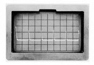
Figure 2-22. 1 μs markers at 50 meters/Div; POLY dielectric.
