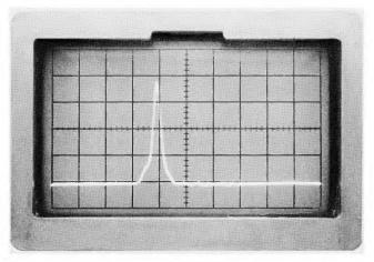
Figure 2-7. "Foot" at beginning of impulse indicating R347 set too far counterclockwise.
