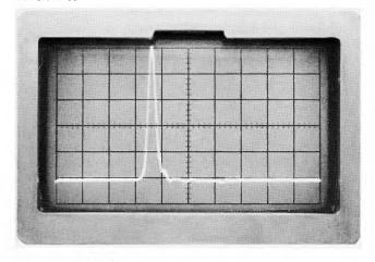
Figure 2-8. R347 adjusted clockwise until "foot" barely but completely disappears.
