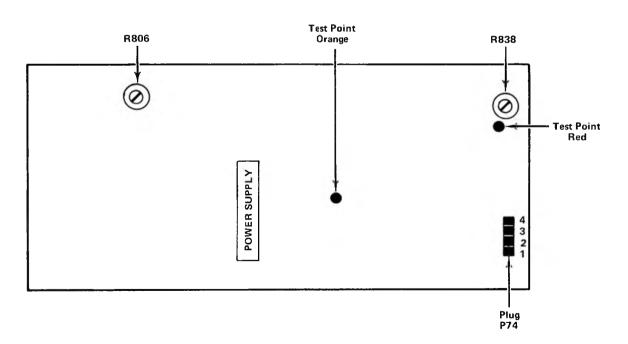
Figure 2-1. Power Supply circuit board showing only test points and adjustment potentiometers. The board is located near the rear of the 1501.
