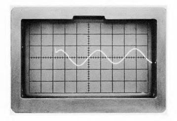
Figure 2-19, 50 ns markers at 5 feet/Div properly positioned for setting of 000 on the START POINT control.
