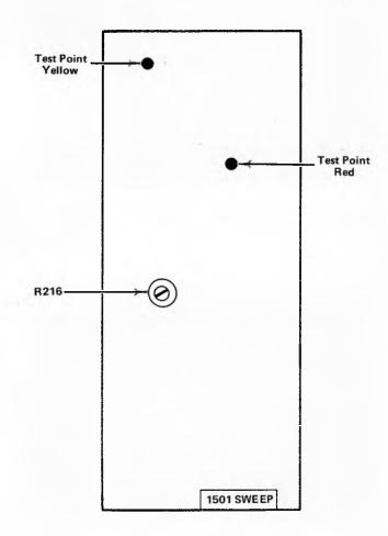
Figure 2-29. Sweep circuit board. Located behind CABLE dielectric switch.
