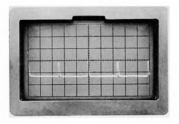
Figure 2-20. 5  $\mu$ s markers at 200 meters/Div; POLY dielectric.
