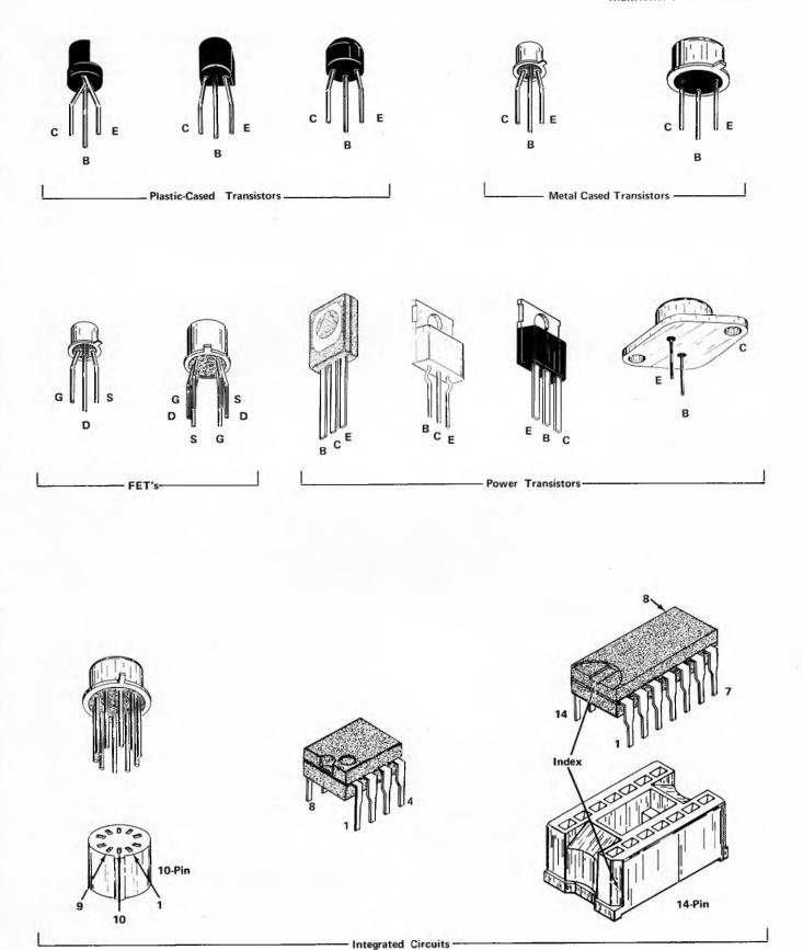
Fig. 3-2. Transistor and Integrated Circuit Lead Configuration.
