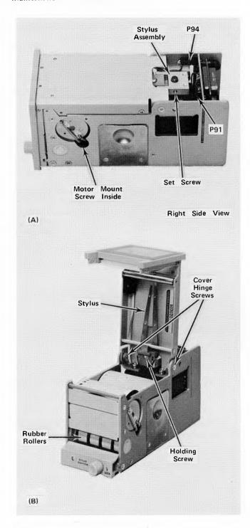
Fig. 3-4A and B. Location of chart recorder components.
