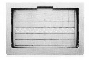
Figure 2-14. 0.1  $\mu$ s markers at 50 feet/Div; 0.81 FOAM dielectric.
