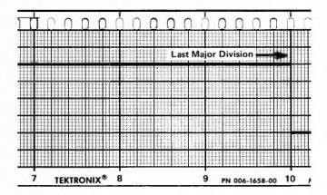
Figure 2-30. Indication of proper adjustment of R216 if paper is properly installed.
